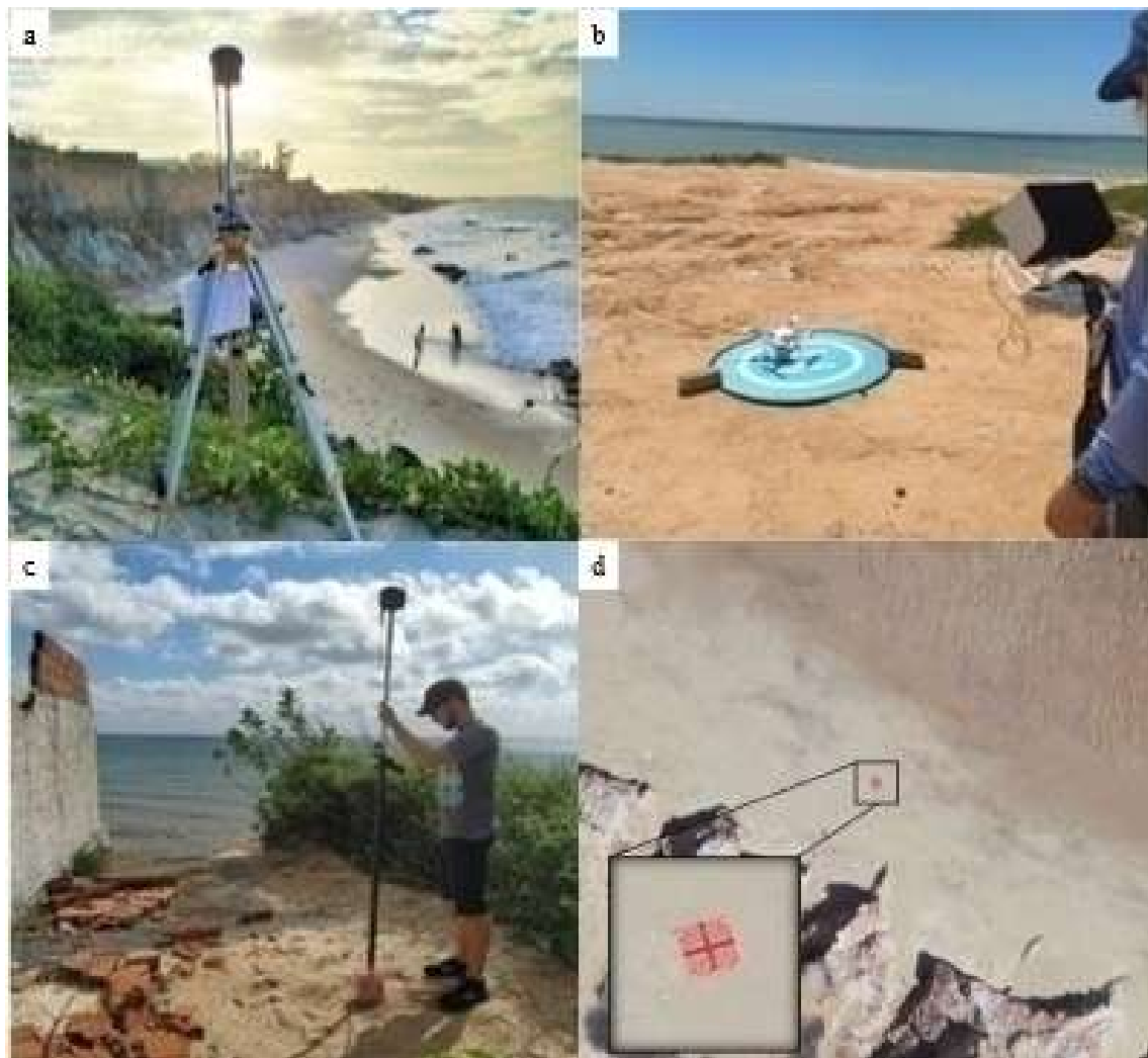
Figure 2 - GNSS-RTK Survey and Unmanned Aerial Vehicle UAV. a) GNSS-RTK base antenna; b) UAV Phantom 4Prov2; c) Fixed points on the cliff top; d) Control points on the beach face.
