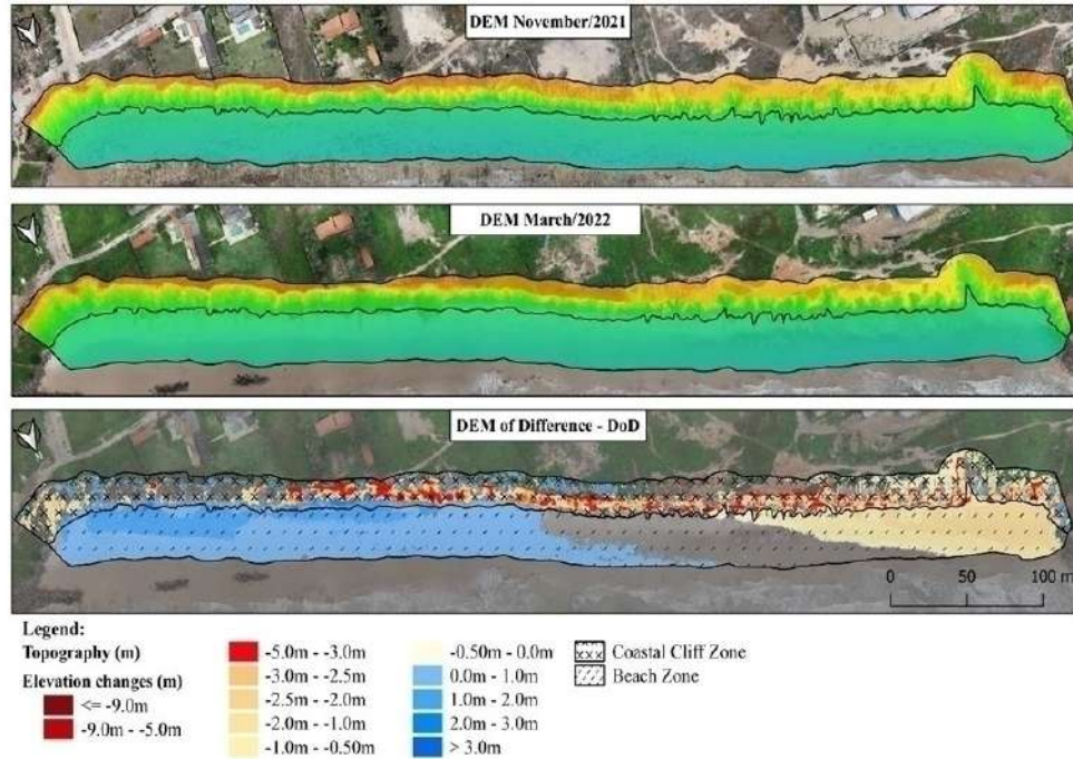
Figure 5 - Changes in elevation and volume recorded in the November/2021 and March/2022 UAV surveys.
