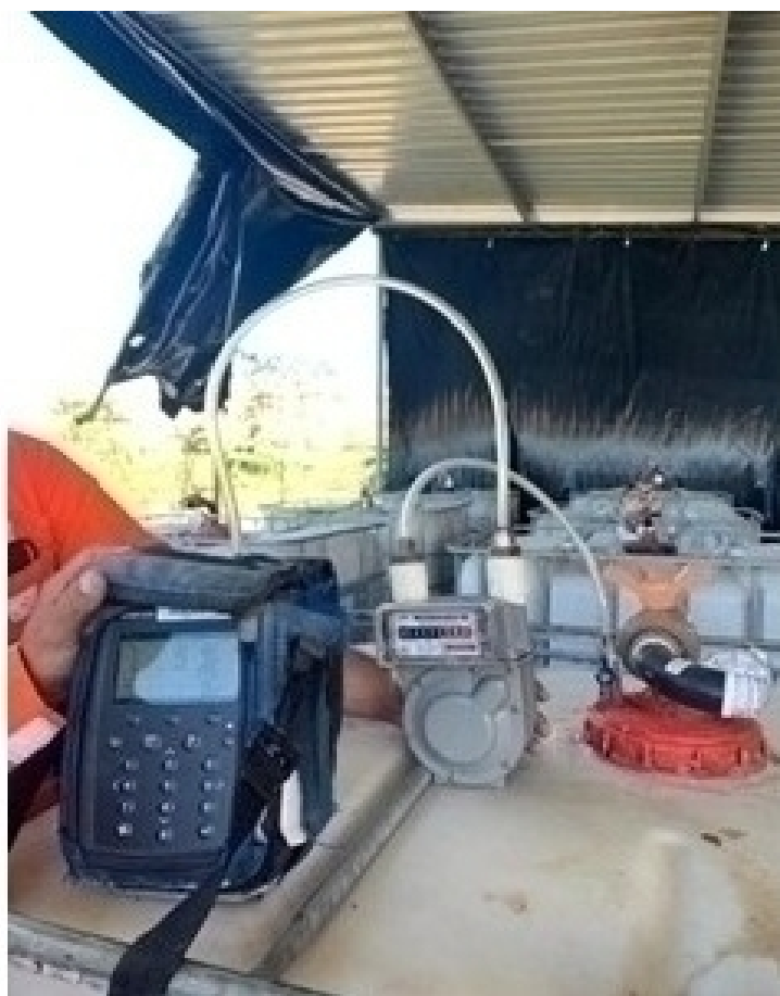
Figure 5 - Measurement of gas flow and composition in the reactors installed at GNR/ASMOC. Source: The authors (2024). Statistical analysis.
