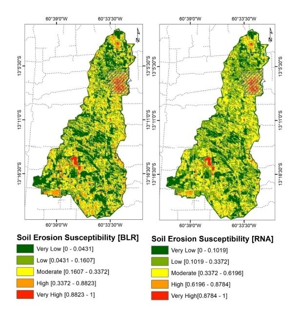
Figure 3 – Map of susceptibility to soil erosion of the Sete Voltas River Sub-basin - Binary Logistic Regression Model [BLR] and Artificial Neural Network [ANN].
