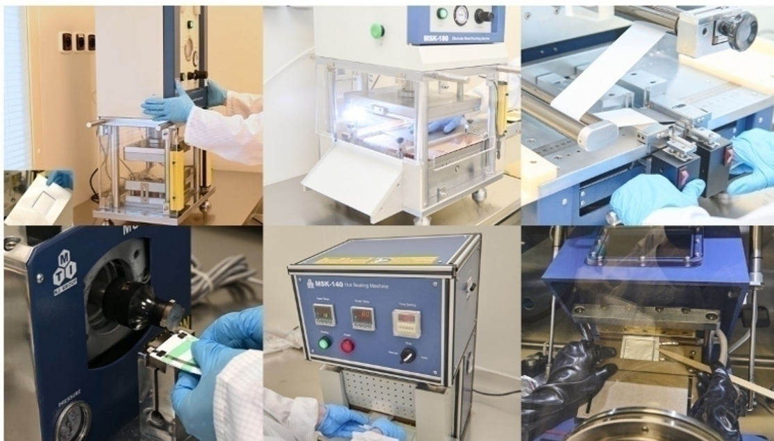
Figure 5 - Laboratory-scale pouch for cell assembly. From left to right, the first step is pouch formation, the second is electrode cutting, followed by electrode stacking and ultrasonic welding, followed by heat sealing, and the last step is vacuum sealing. Source: Image courtesy of the Centre of Polymer Systems, Tomas Bata University in Zlín, Czechia (2024).
